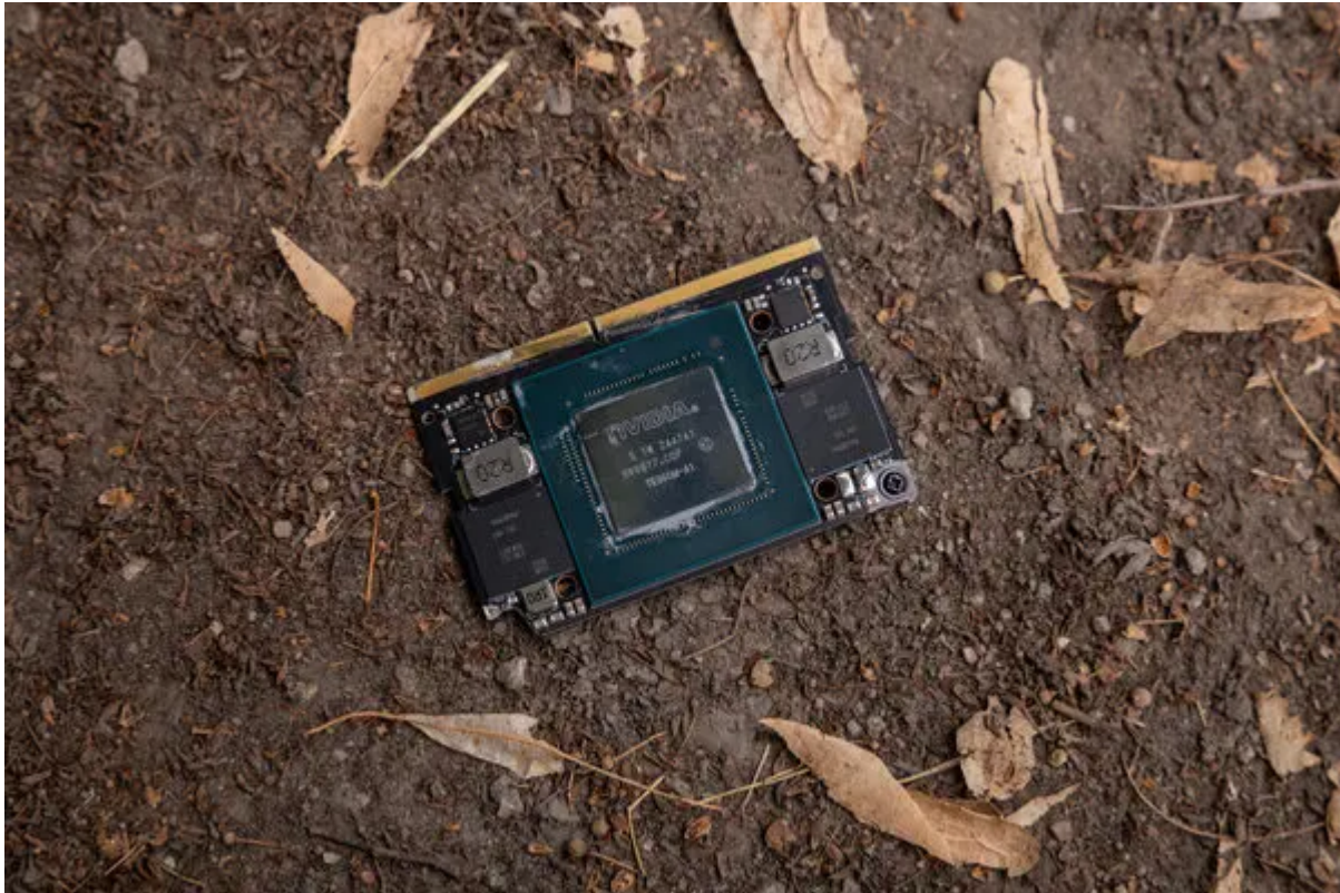
An Nvidia Jetson Orin module used in the Molniya drone.
